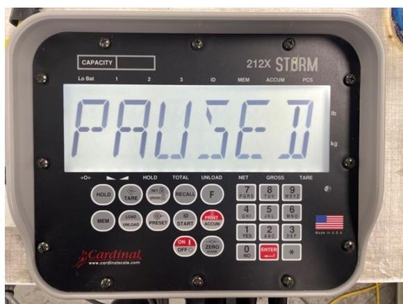
21. The process may be paused during unload by pressing the decrease switch on the spout. By pressing the decrease switch again the operation will be canceled or by pressing the increase switch the operation will be resumed at the point it was at when it was paused.
