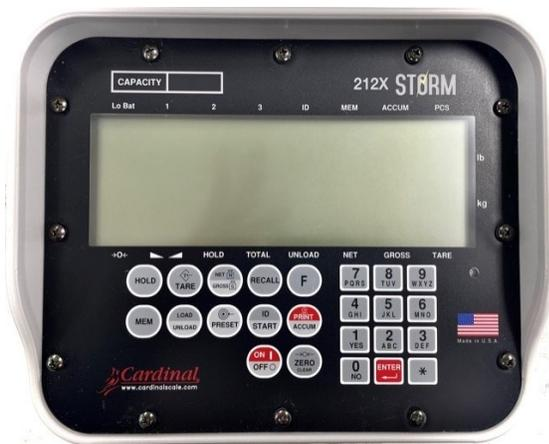
1. Turn on scale indicator by pressing the **ON/OFF** button.
