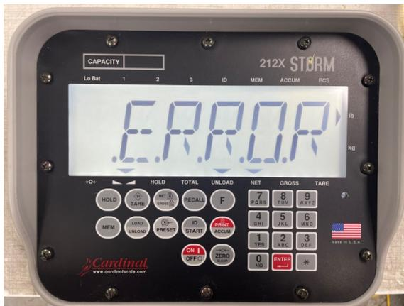
24. Press the increase switch to start a new cycle. If the tare weight was entered correctly the scale will show "ERROR" on the screen if there is not enough seed left to unload the desired amount.
