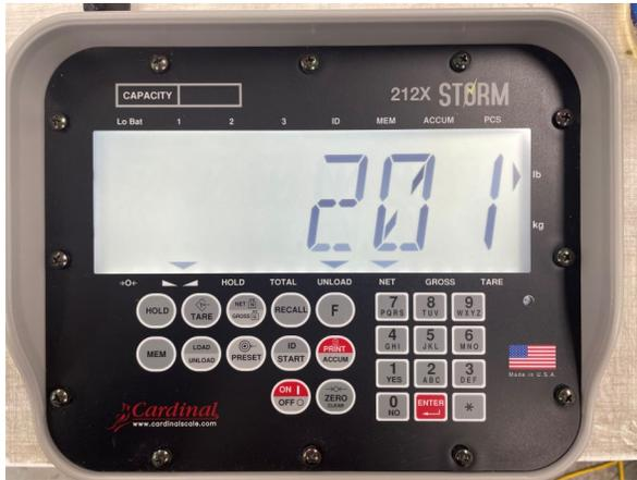
23. The scale will show actual seed unloaded by pressing the decrease button on the spout after the scale shows "DONE" on the screen.
