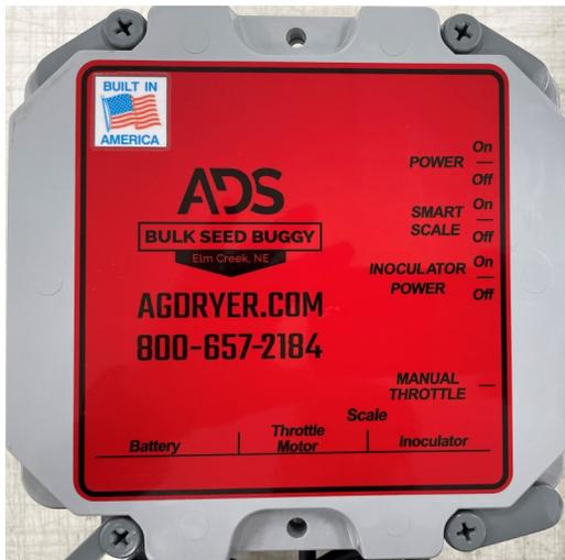
11. Turn on the **SMART SCALE** switch on the seed tender control box.
