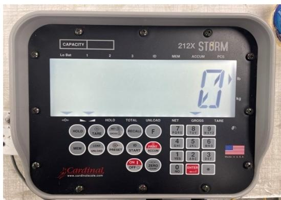
3. **Only** zero the scale if the tender is unloaded by pressing the **Zero/Clear** button. Scale head will read “0”. **Do Not Zero** if tender is loaded with seed.
