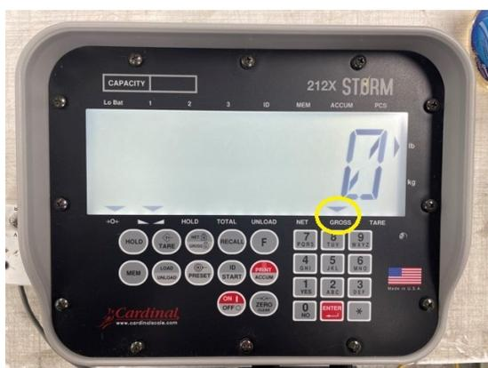
2. Check that the scale is in the **GROSS** mode. Press the load/unload button if necessary. Unload annunciator must be off. If the net annunciator is still on then Press the net/gross button to go to the gross mode.
