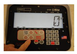
6. Switch to the unload mode by pressing the **LOAD/UNLOAD** button.
