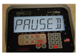
14. The process may be paused during unload by pressing the decrease switch on the spout. By pressing the decrease switch again the operation will be canceled or by pressing the increase switch the operation will be resumed at the point it was at when it was paused.
