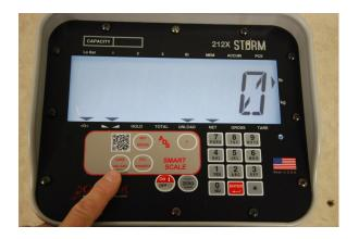
2. Check that the scale is in the load mode. Press the load/unload button if necessary. Unload annunciator must be off. If the net annunciator is still on then Press the net/gross button to go to the gross mode.
