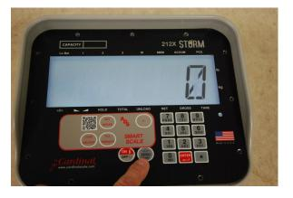
3. Zero the scale by pressing the **Zero** button and the scale will read "0".
