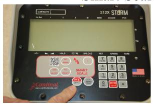
1. Turn on scale indicator by pressing the **ON/OFF** button.
