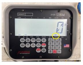
2. Check that the scale is in the **GROSS** mode. Press the load/unload button if necessary. Unload annunciator must be off. If the net annunciator is still on then Press the net/gross button to go to the gross mode.
