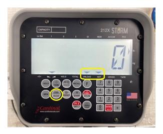
6. Switch to the unload mode by pressing the **LOAD/UNLOAD** button.
