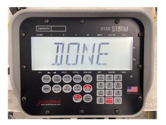
22. When the operation is finished The scale indicator will display DONE.
