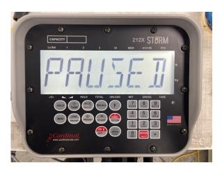
21. The process may be paused during unload by pressing the decrease switch on the spout. By pressing the decrease switch again the operation will be canceled or by pressing the increase switch the operation will be resumed at the point it was at when it was paused.
