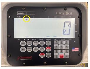
20. Start the unload process by pressing the increase switch on the end of the spout. The scale will now unload the desired amount of seed.
