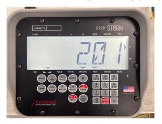
23. The scale will show actual seed unloaded by pressing the decrease button on the spout after the scale shows "DONE" on the screen.
